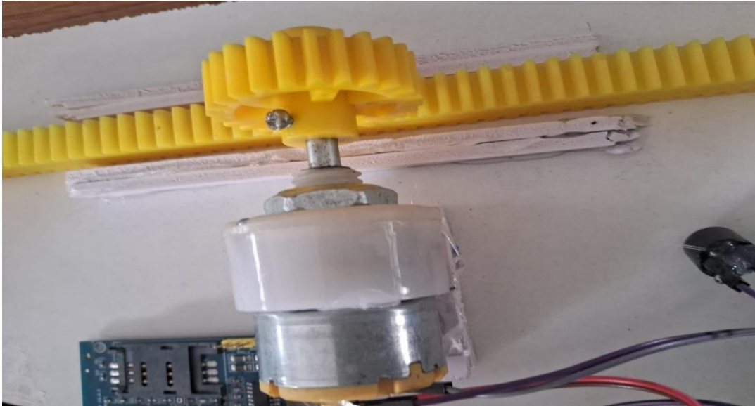
Fig.7.AUTOMATIC DAM GATE CONTROL MECHANISM
