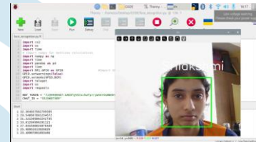
Fig. 4: Real-time LBPH-based face recognition.
