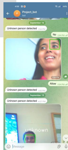
Fig. 6: The cabin owner received a Telegram notification with the taken image .
