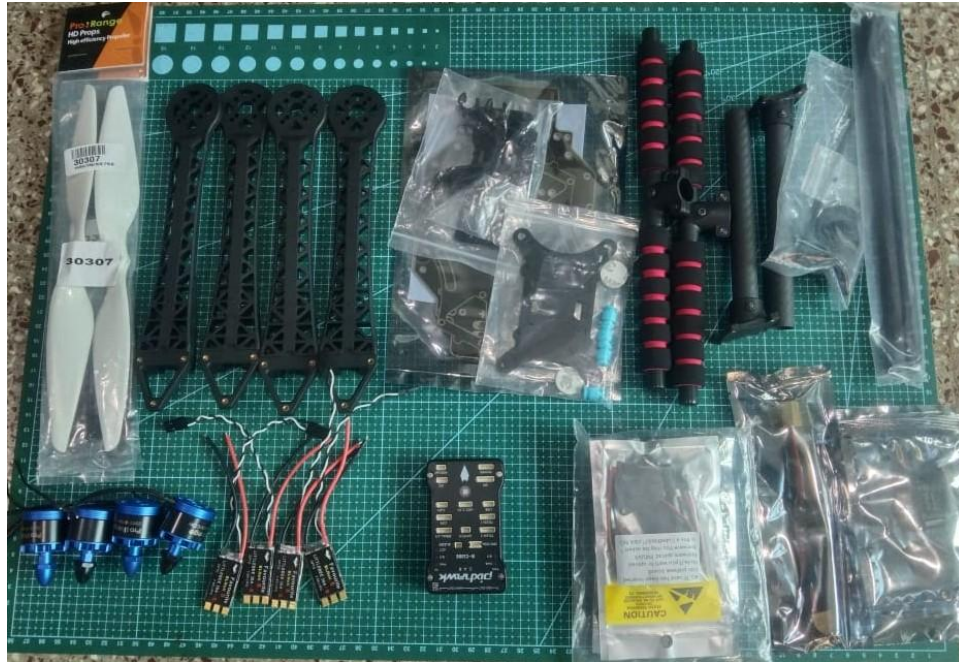
Fig. 5: Complete UAV Hardware Components used in the Proposed System
