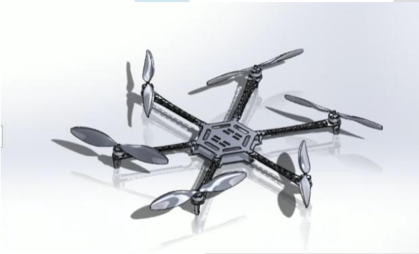
Fig. 1. SolidWorks CAD assembly of the full hexacopter frame (800 mm diagonal, six rotors).
