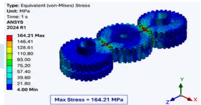
Equivalent (von-Mises) Stress of Actuation Gears
