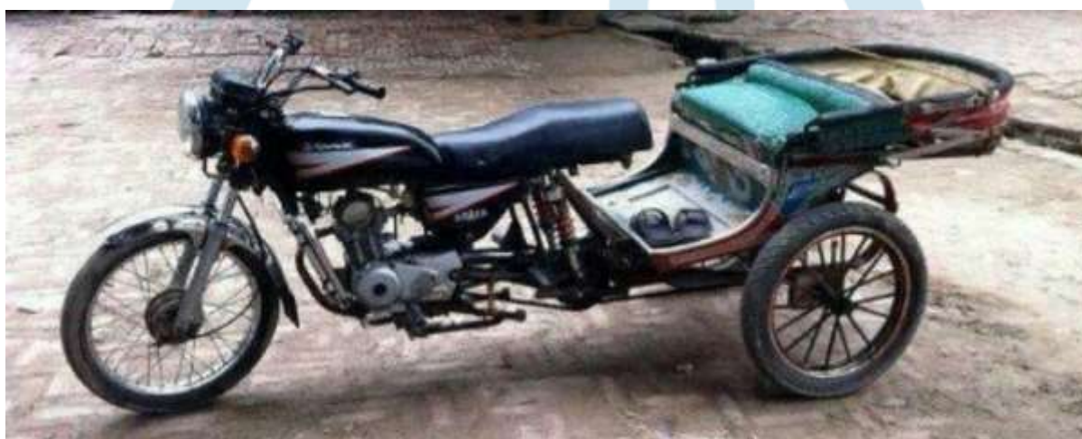
Fig 3: A bike attached to rickshaw seat
